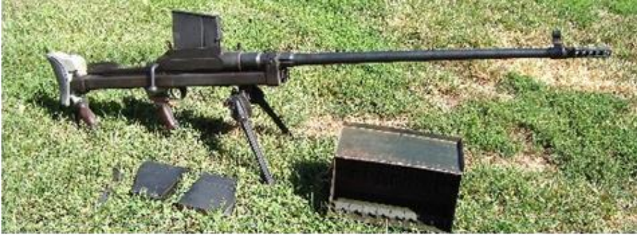
Fig. 4. Boys 13.97 mm calibre anti-tank rifle (courtesy: http://weaponsman.com )
