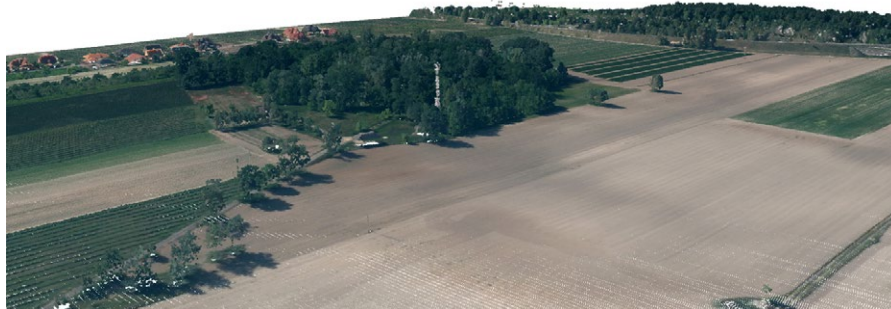
Fig. 11. A cloud of points for an ISOK Project. Displayed using real colours assigned on the basis of aerial photographs
