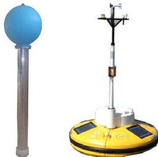
Fig. 6. Sonobuoys used for sonar dataset acquisition: a) designed sonobuoy, b) oceanographic sonobuoy.
