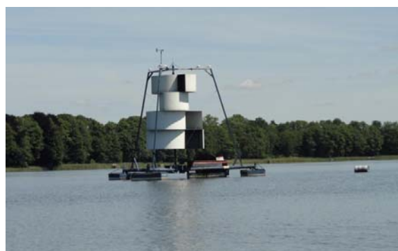
Photo 1. Wind-driven pulverising aerator (photo A. Bryśiewicz)
