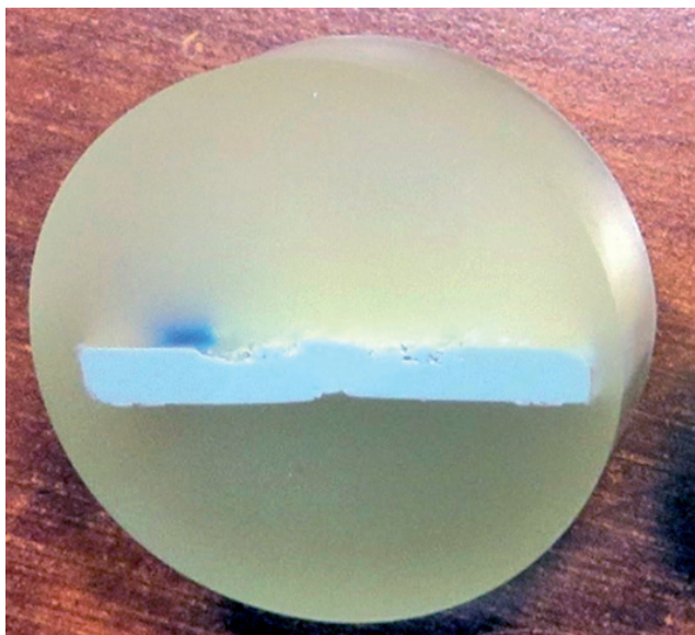
Fig. 8. Sample prepared for microstructure analysis
