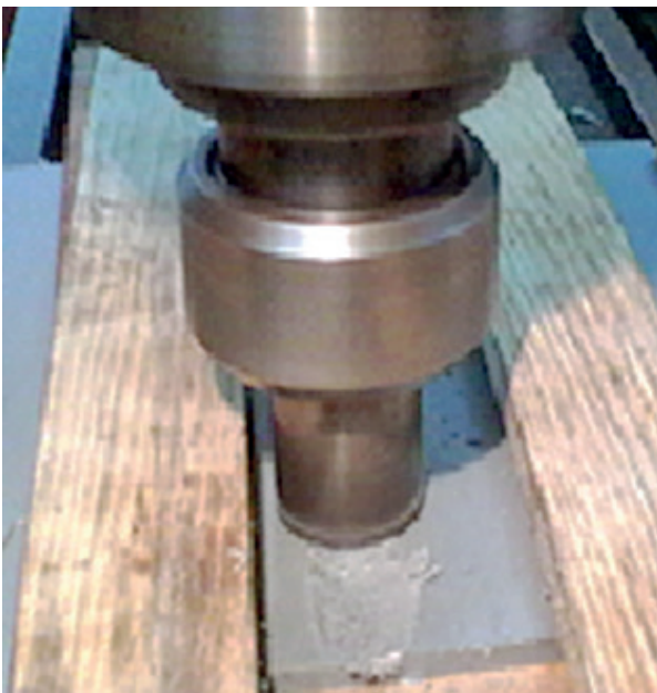
Fig. 2. FSW process of the PP sheets
