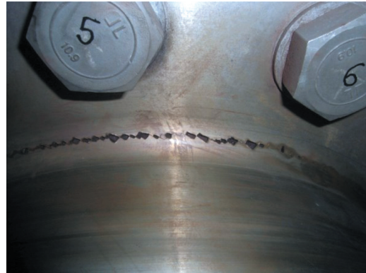
Fig. 2. Cracks in circumference with crushing [1]
