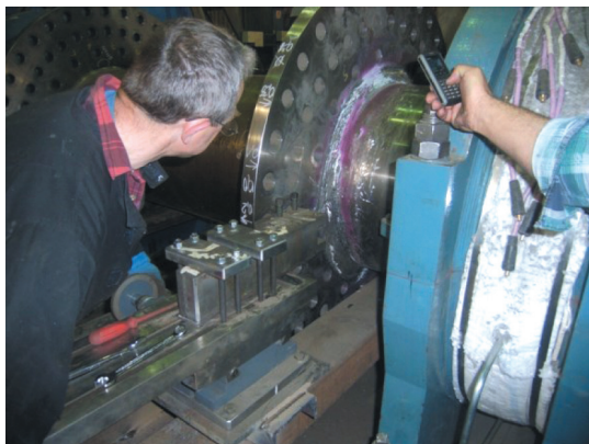
Fig. 9. Machining of shaft after welding to render proper curvature radius for part of shaft [1]
