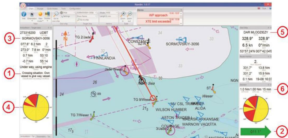
Fig. 2. NAVDEC in action: real screenshot from the NAVDEC pilot test at sea on the 'Dar Młodzieży', showing main components
