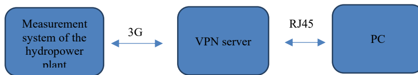
Figure 2. The structure of the master communication system
