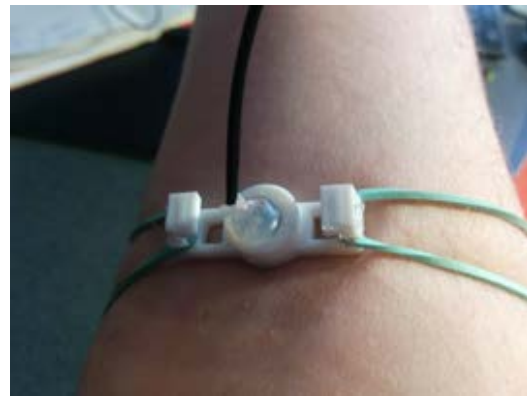
(b) Photograph of mechanomyographic probe
