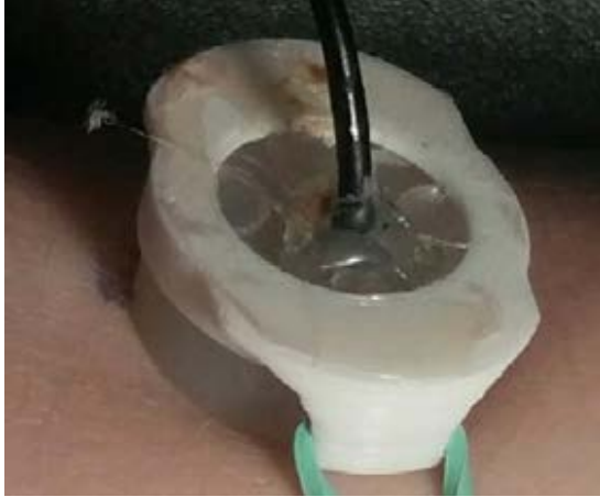
(b) Photograph of silicone-based mechanomyographic probe
