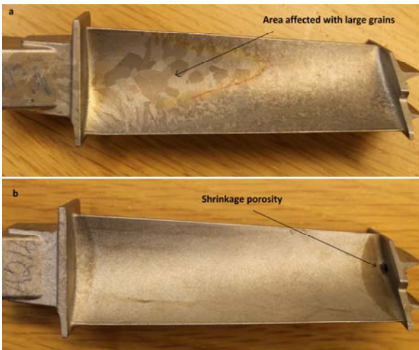
Fig. 1. Common defects in casting of turbine blades
