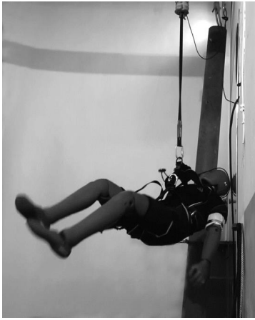
Fig. 5. Collision of the dummy with the vertical structural element for a full body harness with a thoracic attachment point
