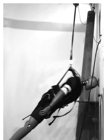
Fig. 4. Collision of the dummy with the vertical structural element for a full body harness with a dorsal attachment point
