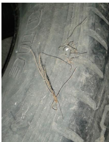
Fig. 2. Defective tire No. 2. Visible fragments of wires from the damaged belting, which pierced the side wall of the tire.
