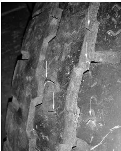
Fig. 1. Defective tire No. 1. Visible fragments of wires from the damaged belting, which pierced the tread of the tire.
