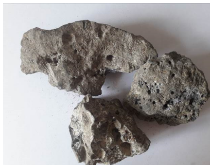
Fig. 2. Aggregate based on open-hearth slag
