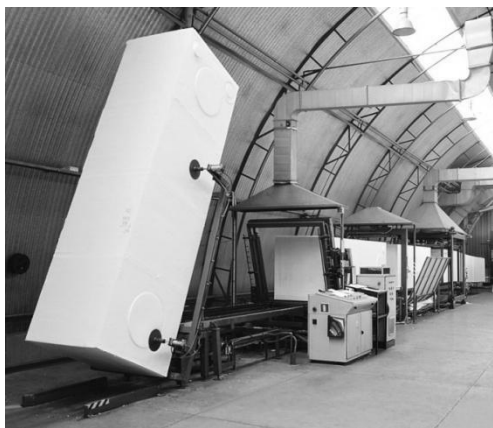
Fig. 3. The line to cut polystyrene.
