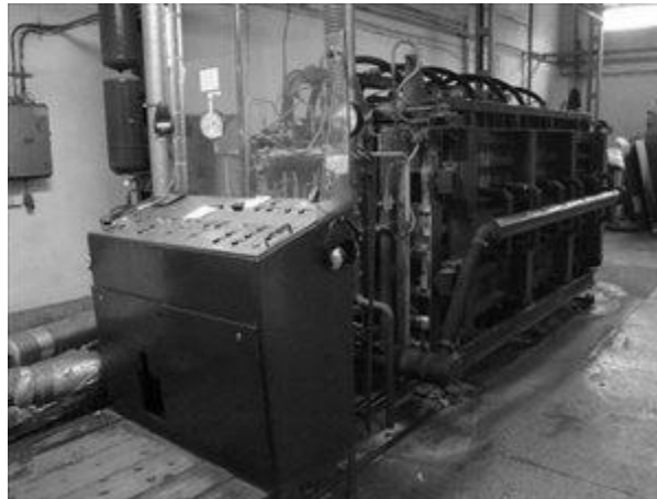
Fig. 2. The machine for forming blocks of polystyrene.
