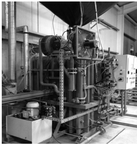
Fig. 1. Machine for frothing of polystyrene with dryer.
