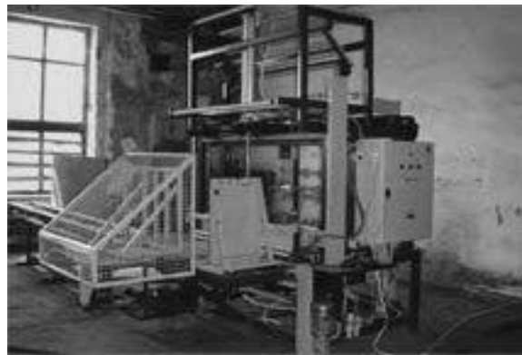
Fig. 4. The plates packaging machine with feeder.
