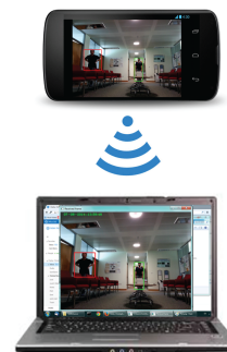
Fig. 1. The outputs from the smartphone application and desktop server when the Wi-Fi capability is enabled and moving objects are detected. When there is no moving object there is a blank screen and a message, 'no motion detected'.
