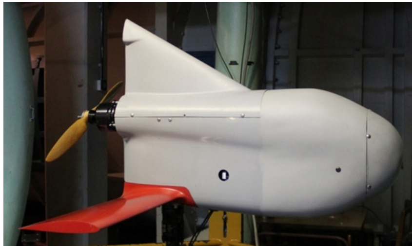
Fig. 7. The pusher propeller of ILX-32 MOSUPS investigated in the wind tunnel
