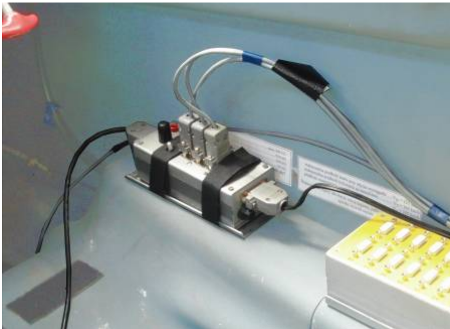
Fig. 4. Photo of measuring system mounted in the PW-6 glider
