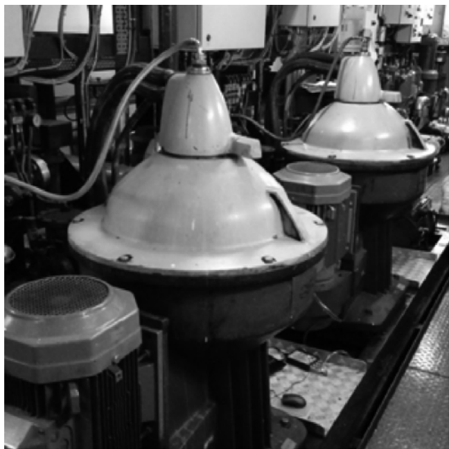
Figure 1. Marine Fuel Separators Alfa Laval SA 861.
