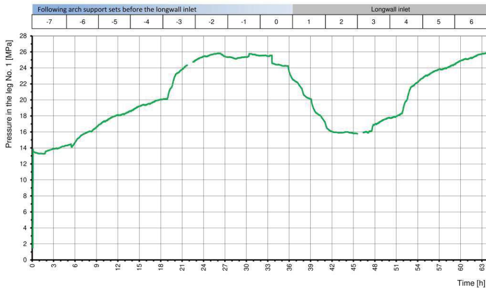
Fig. 8. Course of pressure in the measurement leg [15]
