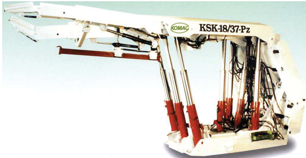
Fig. 4. KSK-18/37-Pz mechanized crossing unit [15]
