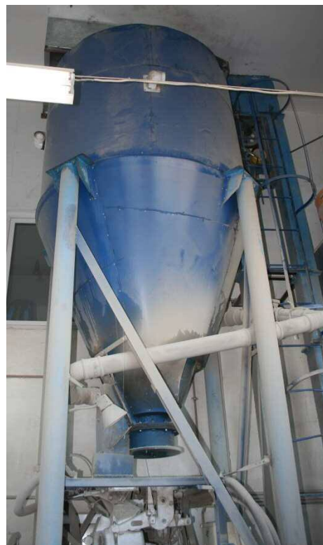
Fig. 2. Mixing line in the following unit: a feed mixer, an intake hopper and a bucket conveyor
