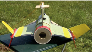
Figure 5. Possible ways of side plate deflection: symmetrical for longitudinal control (on the top left) and asymmetrical for directional control (on the bottom left) [own study].
