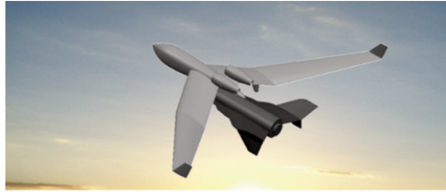
Figure 1. The carrier (light grey) and the rocket-plane (dark grey) flying in coupled configuration [own study].
