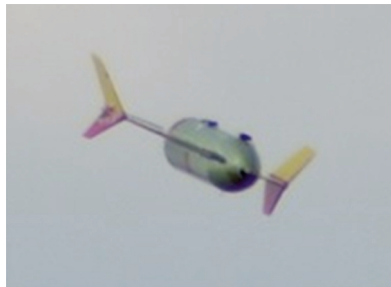
Figure 3. The rocket-plane model: view from a distance. The yellow and red colours were selected to ensure good visibility for the pilot and help to distinguish where the top and bottom of the model are [own study].
