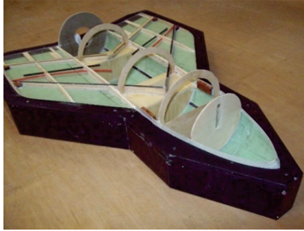
Figure 2. The rocket-plane model during the building process; the inside structure is glued into the composite skin [own study].
