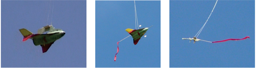
Figure 13. On the left, initial configuration of the holding component (without the ribbon). In the middle and on the right, the modified version of the holding element is shown with the stick and the ribbon [own study].
