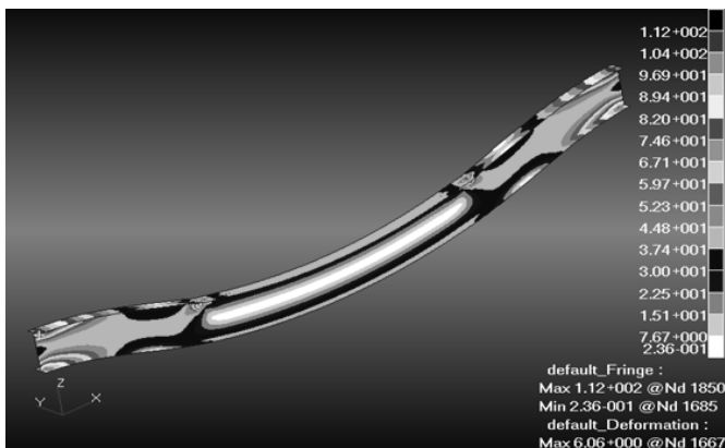
Fig. 3 Reduced stress distribution in the gantry beam according to Huber hypothesis
