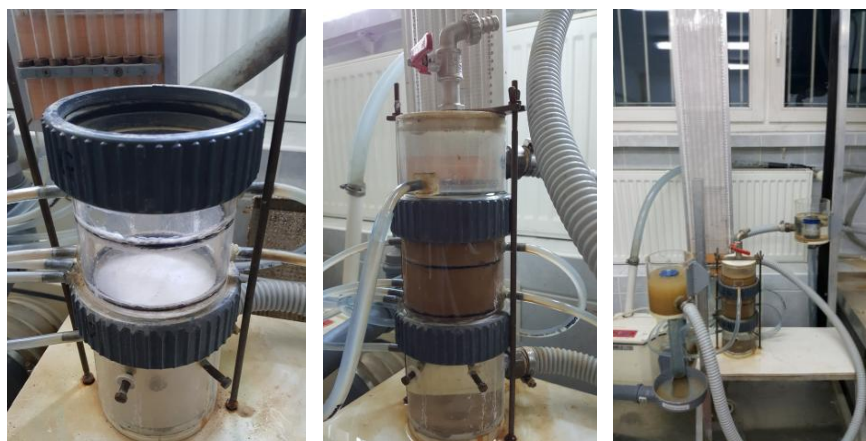
Figure 8. Gradient ratio test device: a) nonwoven geotextile, b) soil and geotextile, c) general view. Source: own photographs.
