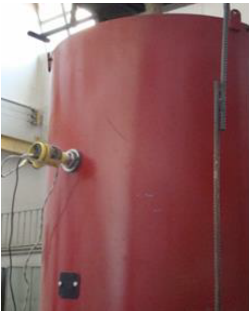
Figure 5: The used pressure transducer.
