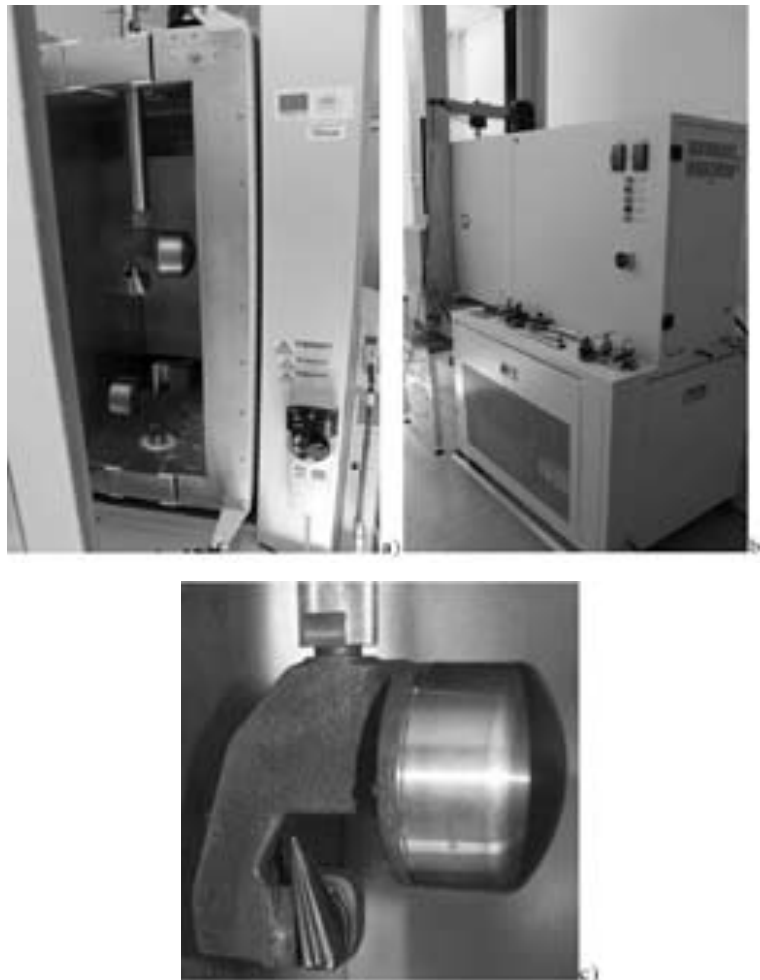
Fig. 8. Universal testing machine (a) with hybrid chamber (b) and detail of special jaw for fibres (c)
