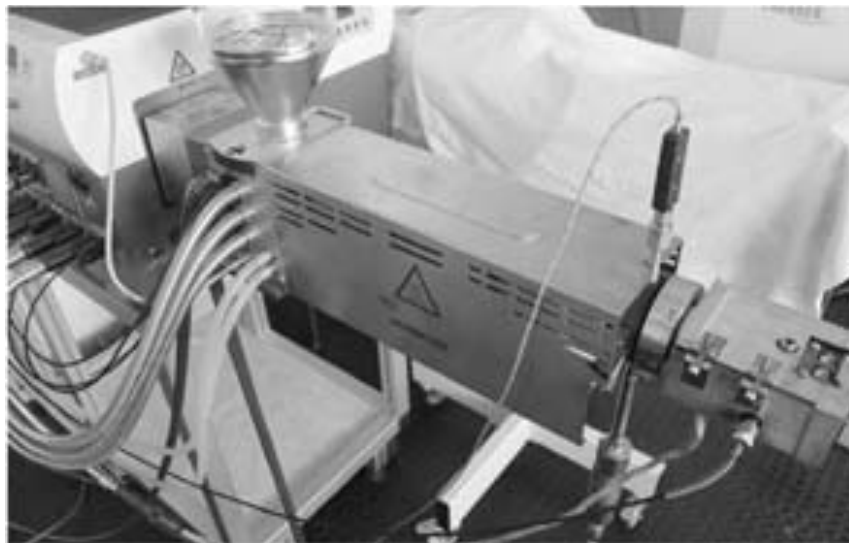
Fig. 7. The measuring extruder of torque rheometer for production of polymers
