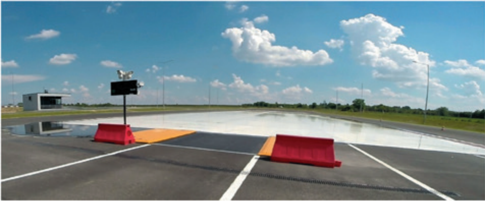
Fig. 6. Rectangular skid pad (the bright area) with a kick plate (the black tetragon), manufactured in Poland by UNIMETAL Sp. z o.o. of Złotów [29]
