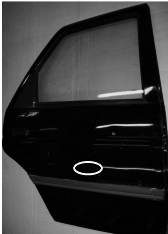
Fig. 1. The tested object – a vehicle door disassembled from the vehicle, with the coating application area marked
