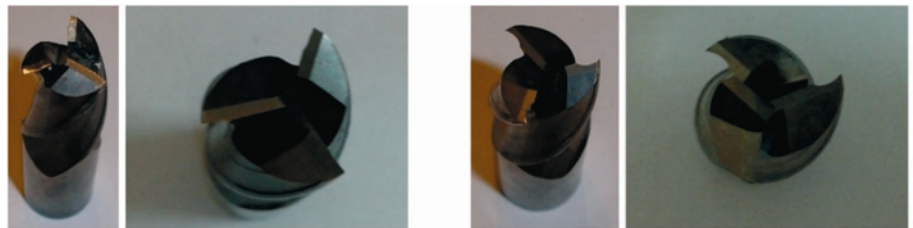
Fig. 4. Three-tooth carbide milling cutter described by an angle of: a) \gamma = 5^\circ , b) \gamma = 30^\circ
