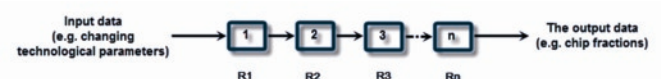
Fig. 1. Example of a reliable structure of a technical object (technological machine) in a series-based system ( R1 \rightarrow Rn – reliability of all elements in the series) [13]
