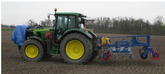
Fig.2. Agricultural tractor with aggregate for pre sawing tillage during field tests [4]
