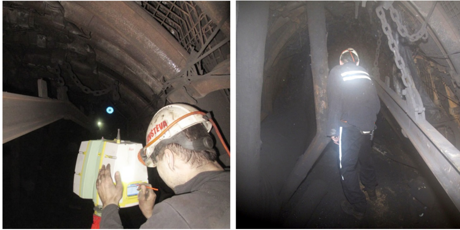
Fig. 9 – Focussing the centre of the target on the scanner display (left); low profile of mining works (right).
