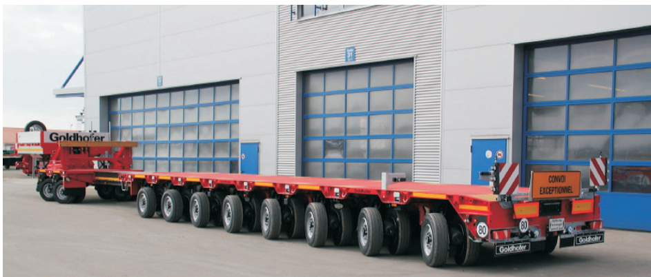
Fig. 9. STZ-P type low-loading semi-trailer
