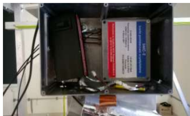
Fig. 1. a) The scintillation detector consisting of a photomultiplier, b), measuring card and the photomultiplier power supply unit
