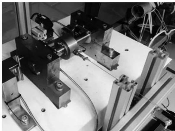
Fig. 1. Test rig used for testing the foil bearing subjected to static loads
