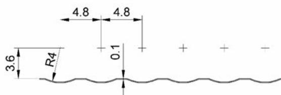
**Fig. 3. The bump foil geometry (dimensions in mm)**
