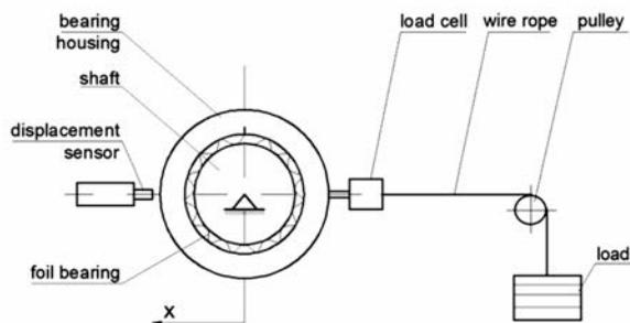
**Fig. 2. Schematic diagram of the test rig**
