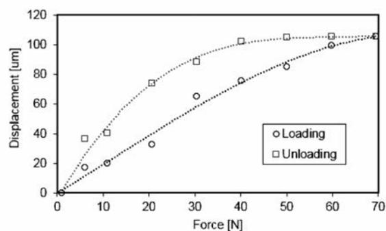
**Fig. 6. Displacement of the foil bearing sleeve vs. static load at the sleeve’s angular position denoted by  $90^\circ$**
