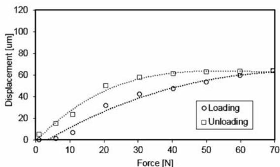
**Fig. 5. Displacement of the foil bearing sleeve vs. static load at the sleeve’s angular position denoted by  $0^\circ$**
