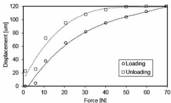
**Fig. 8. Displacement of the foil bearing sleeve vs. static load at the sleeve’s angular position denoted by  $270^\circ$**
