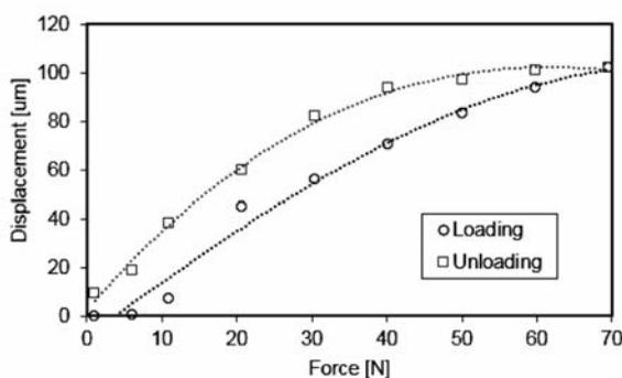
**Fig. 7. Displacement of the foil bearing sleeve vs. static load at the sleeve’s angular position denoted by  $180^\circ$**
