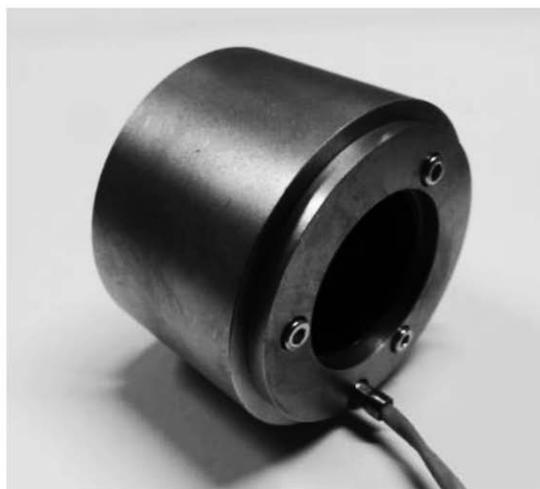
**Fig. 4. The tested foil bearing before and after the assembly**
