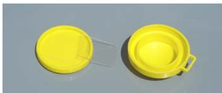
Fig. 1. Opened NRPB-type dosimetric cassette with a CR-39 detector.
