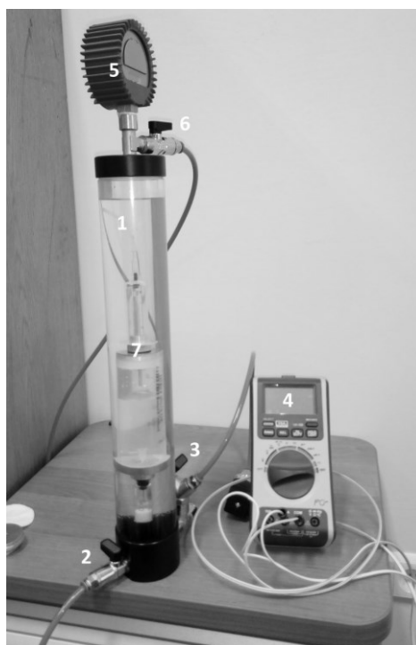
Fig. 2. Experimental stand for research on the concept of autonomous use transport module for transport from the seabed.
