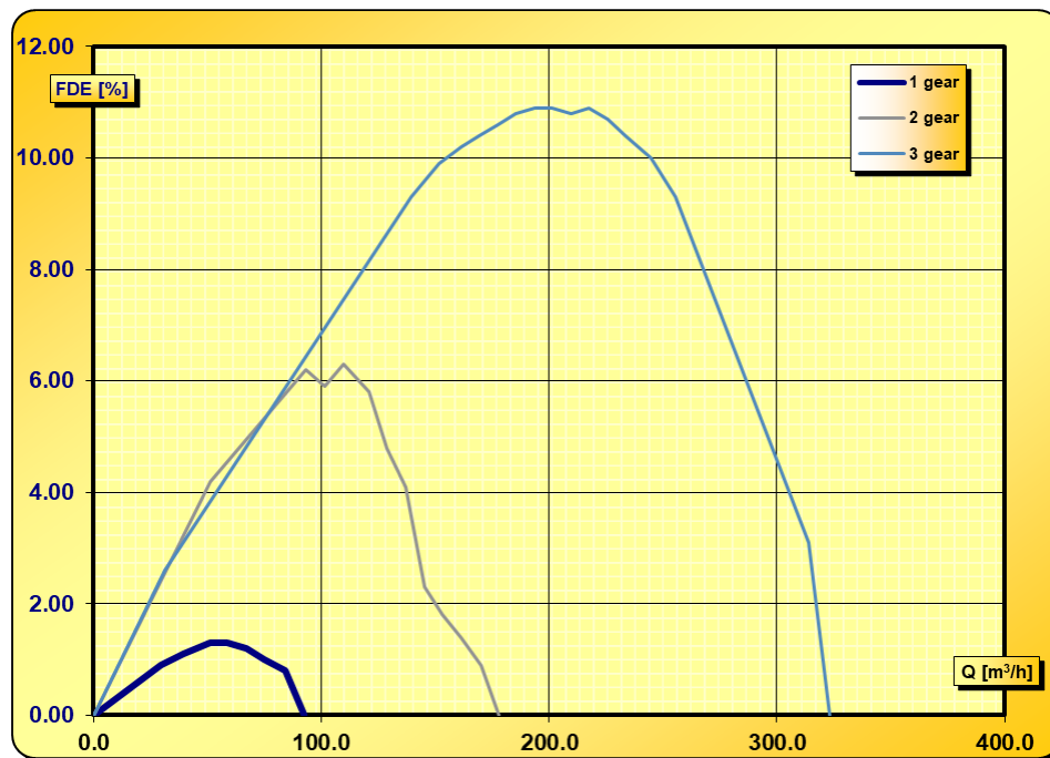
Fig. 5. Fluid dynamic efficiency as a function of air flow rate for the 3 gears of the range hood
