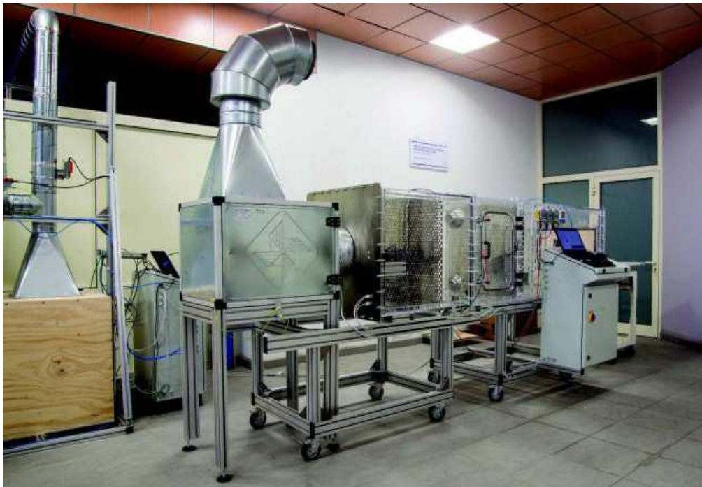
Fig. 2. Flow test bench for fans range hood
