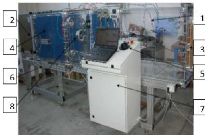
Fig. 3. Functional elements of the test stand: 1 – Calm air chamber, 2 – Booster, 3 – Housing for electric fan under testing, 4 – Observation window, 5 – Variac, 6 – Aluminium profile to support the bench, 7 – Electric panel, 8 – Panel with nozzles
