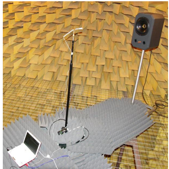
Fig. 6. Overall view of the measurement setup in the anechoic chamber.
