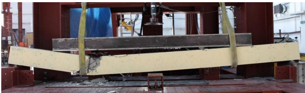
Fig. 3. Failure mode of A-W0 series of beams
