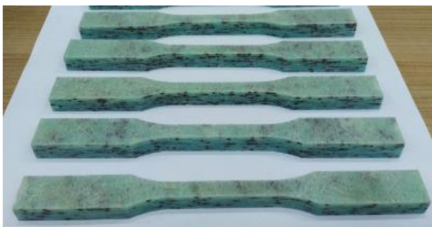
Fig. 7. Test samples cut by water cutting
