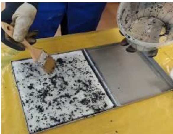
Fig. 6. Manufacture of materials by hand lamination
