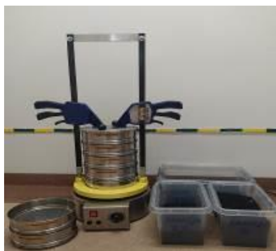
Fig. 4. Sieve shaker LAB-11-200 with separated rubber recyclate fractions
