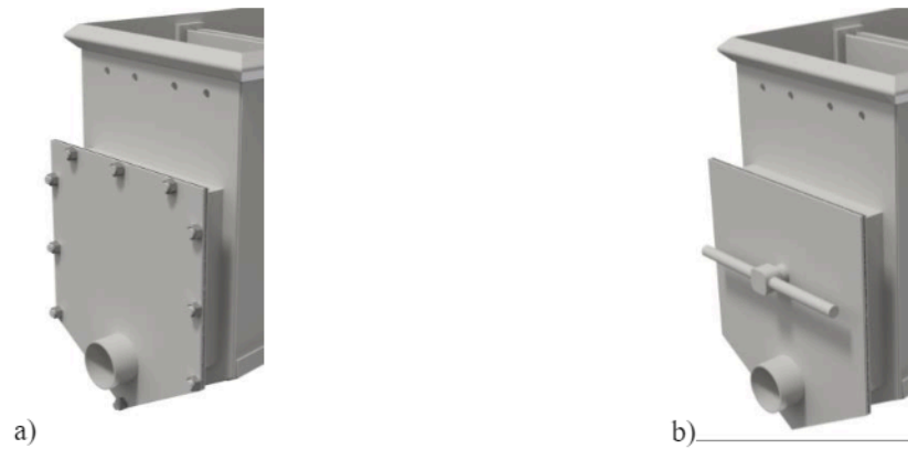
Fig. 14. Tank with a service window: a) using screw connection, b) central pivot bolt
