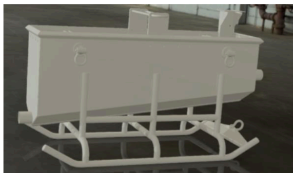
Fig. 16. Base water tank with sliding support frame
