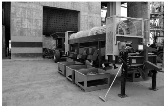
Fig. 12 A drum sorter used in Cement plant in Namibia
