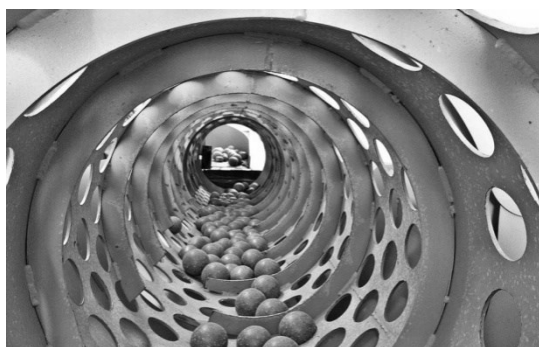
Fig. 13 A view of interior of the drum sorter at work
