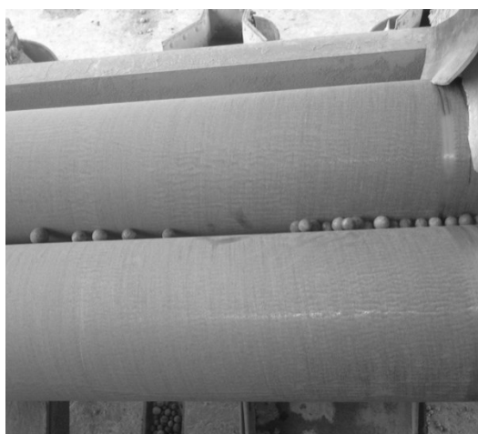
Fig. 7 A view of the phenomenon of mutually moving grinding balls
