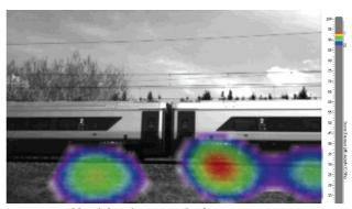
Fig. 3. Sound level distribution in the frequency range 830–885 Hz [autors' elaboration]
