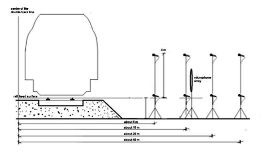
Fig. 2. Intersection of the equipped measurement stand for the field tests [autors' elaboration] [opracowanie autorów]
