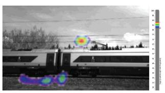
Fig. 4. Sound level distribution in the frequency range 190–2340 Hz [autors' elaboration]
