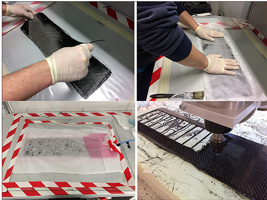
Fig. 8. Procedure for preparing composite parts for tested samples
