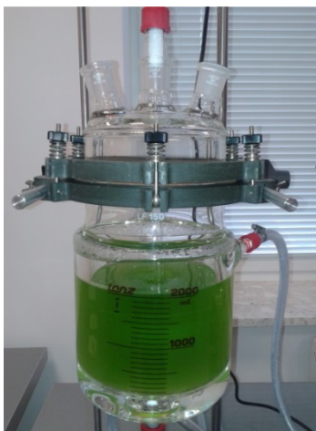
Fig. 3. Laboratory stand for the algae cultivation
