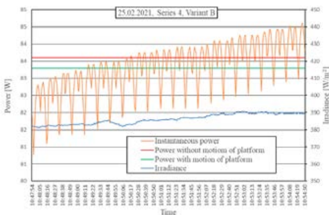
Fig. 23. Change of power and irradiance for variant B in research on 25 February 2021, \tau_c = 20s , series 4
