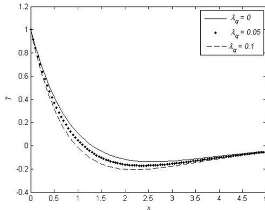
FIG. 10. Variation of temperature  $T$  with distance  $x$  for time  $t = 1.21$ .
