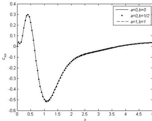
FIG. 5. Variation of stress  $\sigma_{xx}$  with distance  $x$  for time  $t = 0.69$ .
