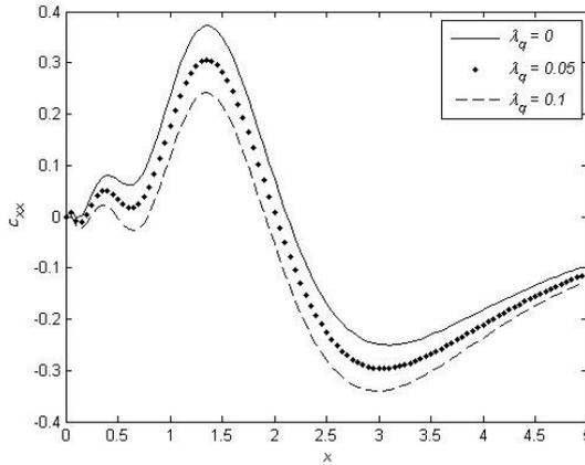
FIG. 12. Variation of stress  $\sigma_{xx}$  with distance  $x$  for time  $t = 1.21$ .
