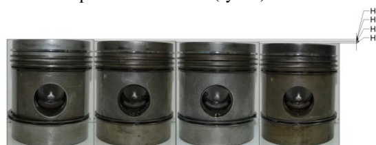
Fig.1. The test engine pistons of various height enabling a change of the compression ratio over the range of \epsilon=17 \div \epsilon=14
