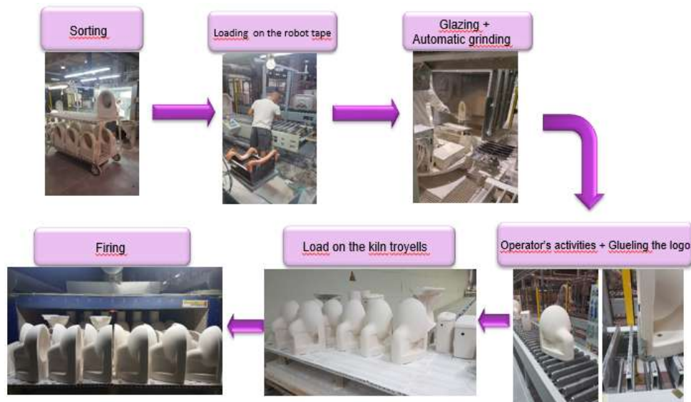
Fig. 5 Actions performed in the Raw Sorting Department after the change (own study)
