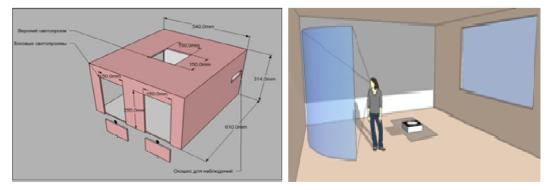
Fig. 2. The model standard room with a vertical window to evaluate the reflected light flowing into the horizontal photocell
