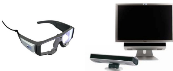
Fig. 1. Example of mobile (left picture) and stationary (right picture) eye-trackers [6]
